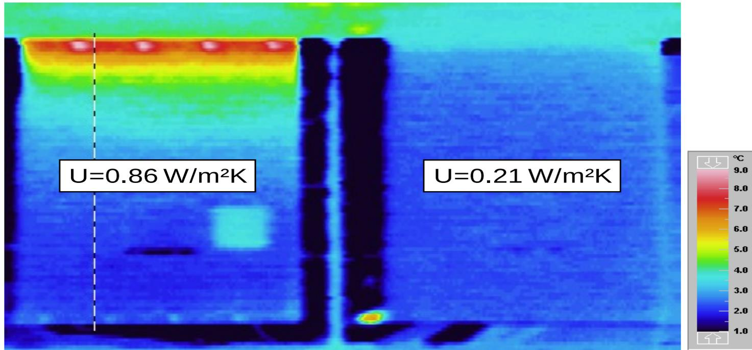
Consequence of good or bad workmanship (theoretical value is  $U=0.16\text{W/m}^2\text{K}$ )
