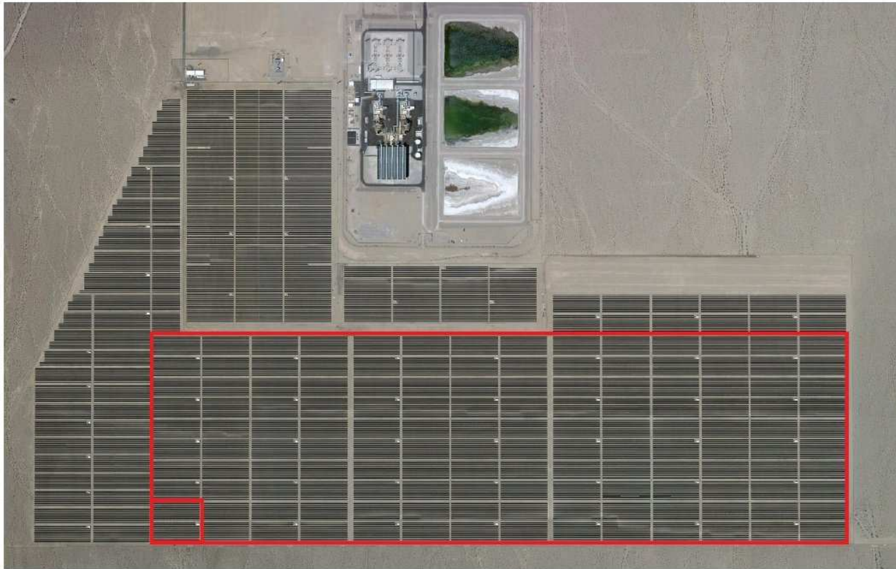
Figure 1: An aerial photo of the Copper Mountain Solar Facility. The small red rectangle indicates the size of a single inverter, which is 125m by 125m. The large red rectangle indicates the 5 by 14 inverters for which we provide forecasts of the power production.
