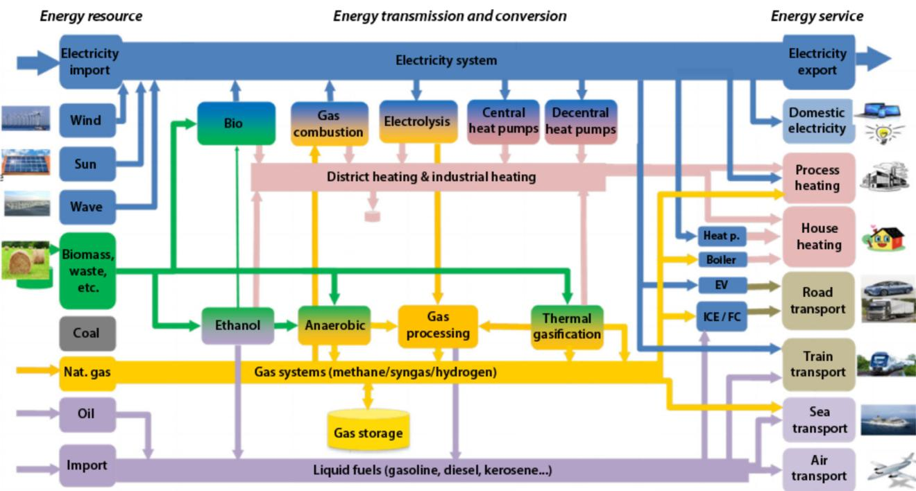
The aim is to optimize the future usage of resources, while delivering the required energy services in a sustainable and reliable way. Figure from Energinet.dk
