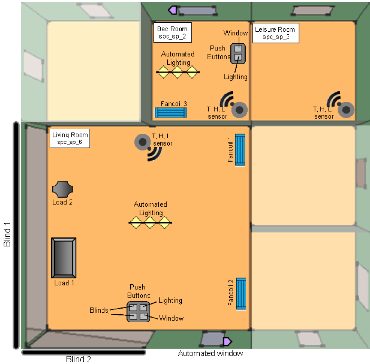
Overview about activated devices inside KUBIK
