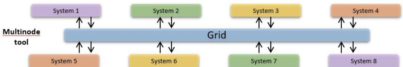
A Multinode tool was used and is a simple method to balance the potential import and export of energy based on the principle that a system can not import more electricity than needed, nor can it import more electricity than available. Therefore, the sum of import and export between systems will always equal zero. Multinode is an add-on to EnergyPLAN
