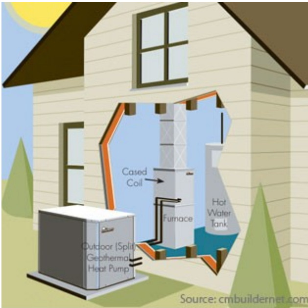
An example of a outdoor dual fuel split unit installation matched with a cased coil
