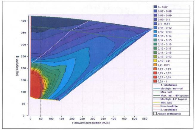
**1The Iron Diagram for Odense CHP station – the relationship between its power output and the heat output. MWe electrical power vertical axis, MWth heat on the horizontal axis**
